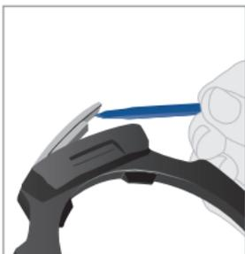
Use the narrow end of the blue removal tool to pick out the grey cover plate. The cover plates vary in size, according to whether the filter guide block has one, two or three slots. Keep the plates safe with the blocks for future use.
