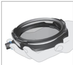
Ease the whole unit into the engaged clip, then snap the second clip into place. Make sure the polariser is secure before attaching the holder to the camera.
