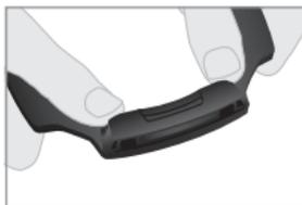
To fit a new filter block, make sure the word LEE faces up and the open side of the block faces outward.
