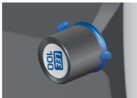
With the blue locking dial in the neutral position, the spring release is pulled out to allow the holder to be attached to the adaptor ring. With the locking dial in this position, the holder can be knocked off the adaptor ring should you catch it in your clothing, for example. This will protect your camera and lens from potential damage.
