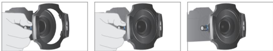
To fit the LEE100 holder to any LEE Filters adaptor ring, first ensure the spring release is in its neutral position, before pulling it to open the holder. Hook the two black teeth into the adaptor ring, then slot in the other side of the holder before letting go of the spring release. The holder will now be fixed in place.
