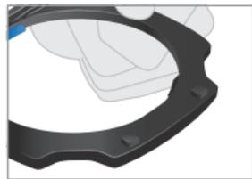
Insert the larger, flat end of the blue tool into the small slot in the middle of the base of the guide block. Push the tool in until you feel resistance. You are not prising the block loose – you are releasing a catch under the block, which holds it in place.
