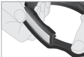
Place the appropriate size of grey cover plate into the open side, making sure it is in the correct orientation, to complete the assembly. Keep all the spare parts somewhere safe, as you will need them should you wish to reconfigure the holder at a later date.
