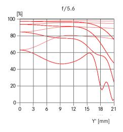
The MTF is indicated at full aperture, at f/2,8 and f/5,6 at long taking distances (infinity). Shown is the contrast in percentage for 5, 10, 20 and 40 lp/mm accross the height of the 35 mm film format, for tangential (dotted line) and sagittal (solid line) structures, in white light. The 5 and 10 lp/mm will give an indication regarding the contrast ratio for large object structures. The 20 and 40 lp/mm records the resolution of finer and finest object structures.
